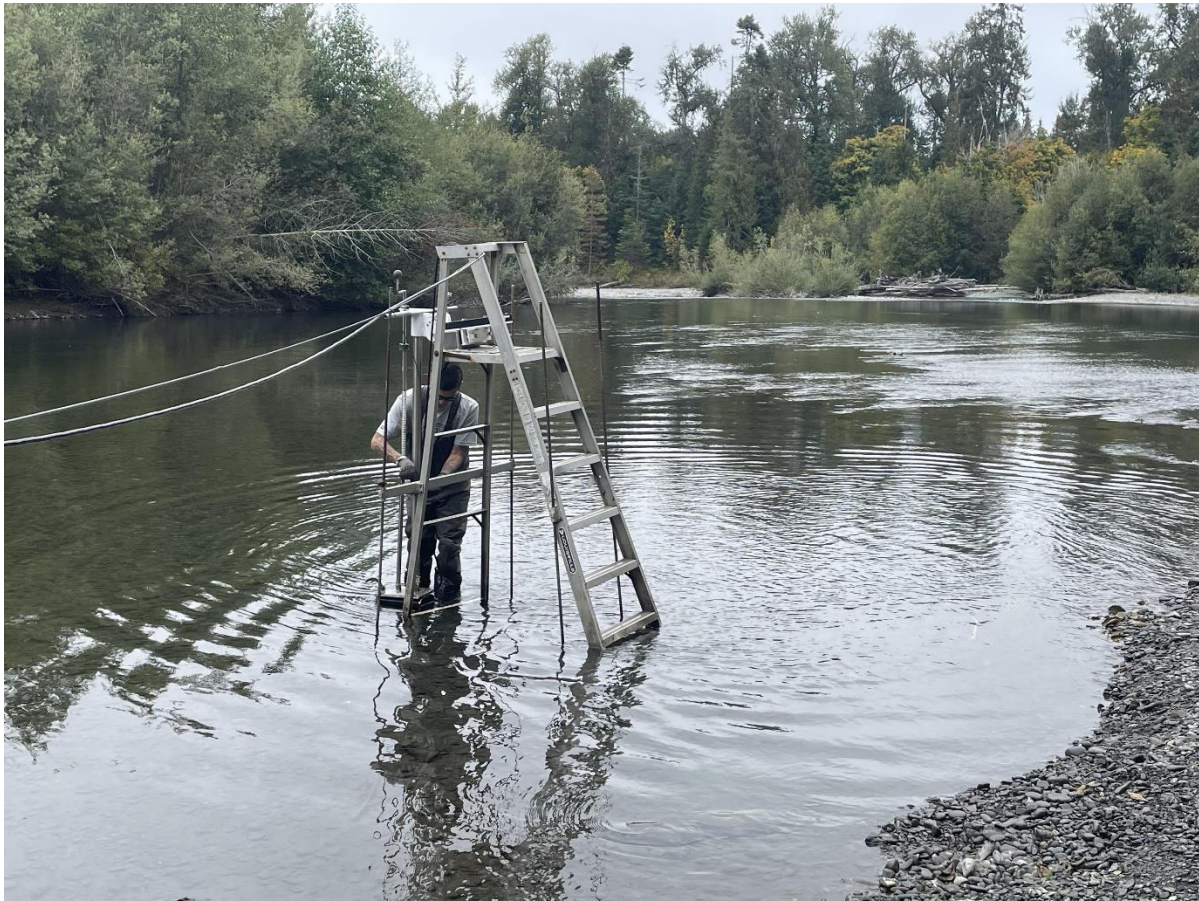
Figure 2. Mainstem SONAR site (formerly referred to as the Old Mainstem). The SONAR is attached to the pole mount which is in turn attached to the ladder.
